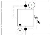
A screw-in, poppet type, direct-acting, cartridge-style hydraulic relief valve. For use as a pressure limiting device for common hydraulic circuit protection.
